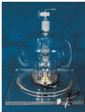
Fig. 3. The prototype kilogram. The only object that has a mass of exactly one kilogram. The prototype kilogram, the last artifact unit of the SI, is kept in a vault at the Bureau International des Poids et Mesures in Sèvres near Paris.
